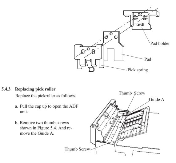
Figure 5.4 Pick Roller replacement
